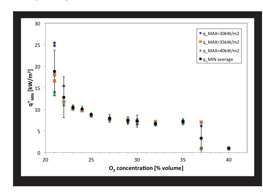
Limiting Oxygen Index (LOI) is the minimum O2 concentration for flame spread.
